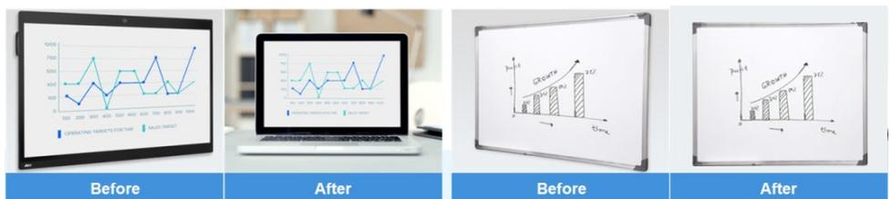
Keystone Correction adjusts the geometry of an image to make it appear rectangular and aligned.
